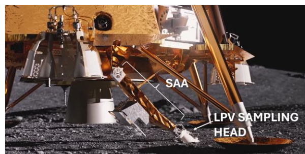
Figure 3. Illustration of PlanetVac Sampling Head deployed to the lunar surface. Image credit: Firefly Aerospace. [2]
