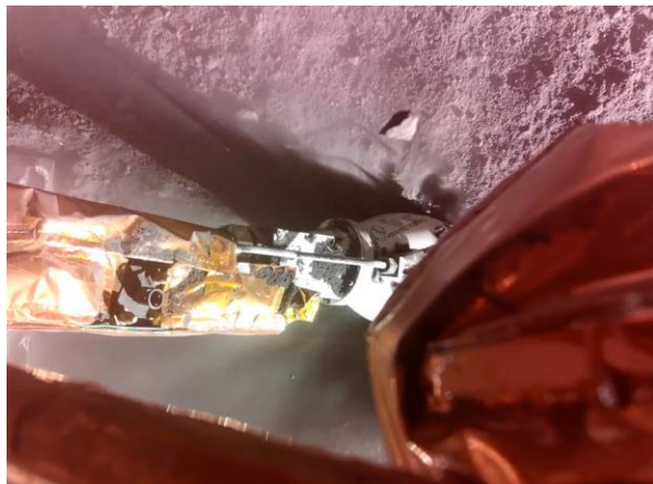
Figure 1: PlanetVac mid-sample capture at Mare Crisium, March 3 rd , 2025. Photo credit: Firefly Aerospace [1]
