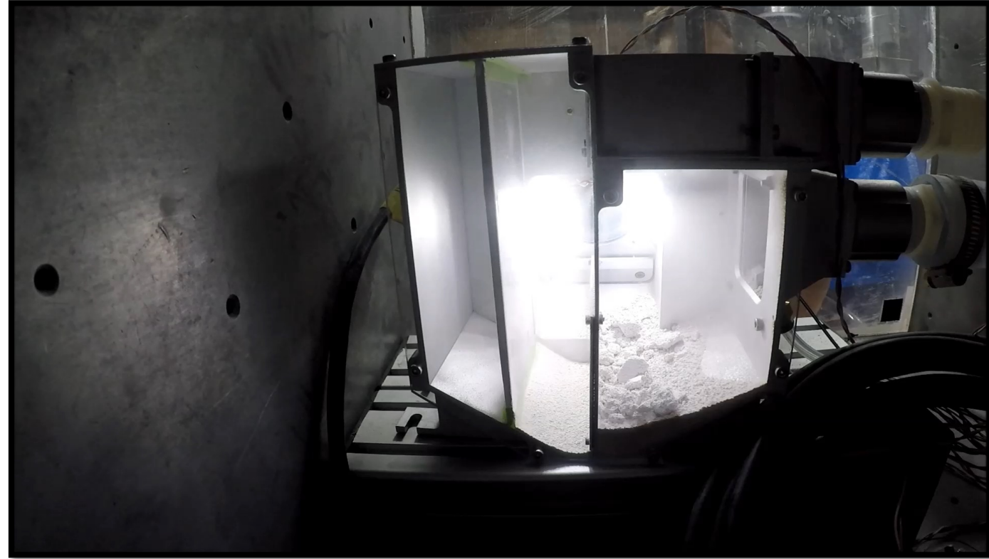
Sample Sieving (Footage from developmental testing)
